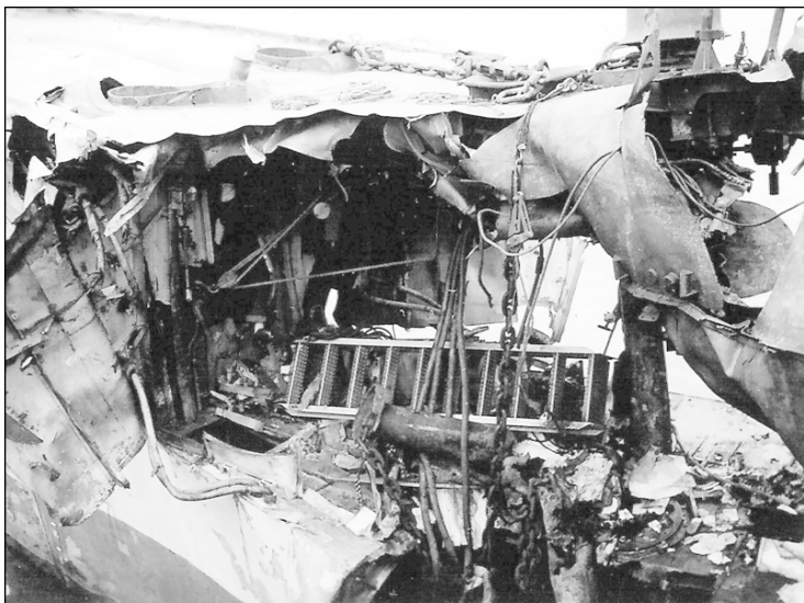
LOOKING THROUGH -- This photo of the port side of the Rodman's bow shows the damage caused by the first kamikaze and his bombs.
